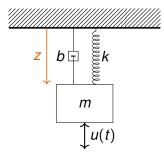
Model with external input u(t)  $\rightarrow$  Linear time invariant system X' = AX + Bu
